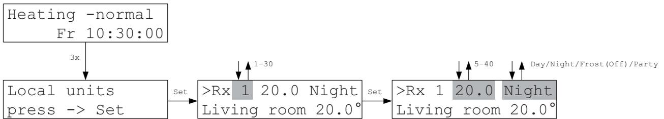
The local units menu allows changing the set temperature and the mode of each local unit from the central unit. The values set manually on the local units are thereby overwritten. For RS local units this is the only means of entering the set temperature.
