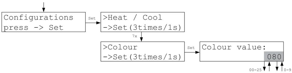
In the Colour menu one of 256 different colours can be set for the display of the ZE central unit (die colours for the displays of the RG / RF local units are set in the units directly).
